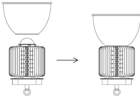
2. Fix the reflector on lamp body and screw tight.
