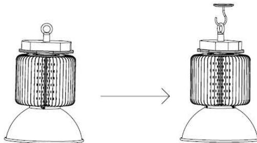
3. Hang up the light on hook and keep stable placement. For safety, make sure the power cables are connected by electricians. The power cord is 0.75-1MM<sup>2</sup> three-core cable wiring, the red is live wire, blue is neutral wire, and yellow is earth wire.
